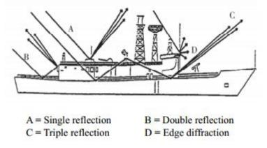
Main scattering mechanisms on naval ships
